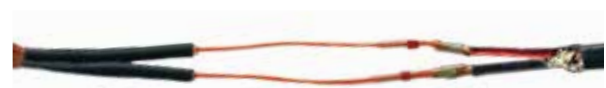
Fig. 3.31: Push the heat-shrink tubing further back and cover with damp cloth before soldering tubes.
