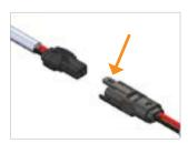
Separate the connectors. **INSTALLATION TIP:** Use caution when disconnecting the LED. There is a small locking tab on the connector that needs to be lifted slightly before the connectors can be separated.
