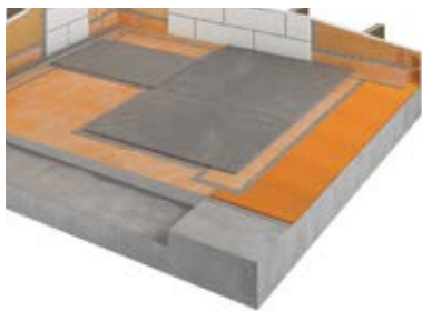
Recess the Shower Floor
