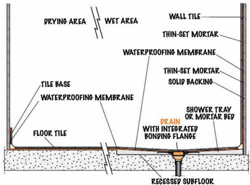
Ideally, the floor will be recessed before installing a sloped mortar bed or prefabricated shower base to allow an even transition at the door threshold. This process can be relatively straightforward in new construction and can also be accomplished in renovations.
