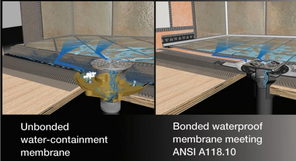
Unbonded water-containment membrane
