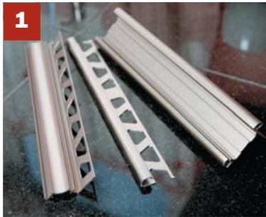
**1.** The first step in using the Schluter edging is to plan the layout. The aluminum profiles need to be fitted together properly. This is not difficult, as there are special inside and outside corner pieces, for example, to join sections together. But it does mean setting up your tile layout and your edging layout before you start the installation
