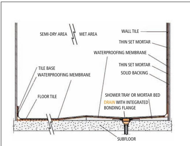
The floor area has been built up over a concrete slab. The floor inside the shower area slopes to a centre drain, and the floor outside the shower area slopes away to the bathroom door.
