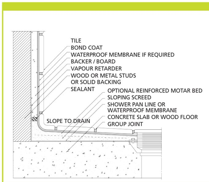
*A shower pan assembly using a two-stage drain.*
