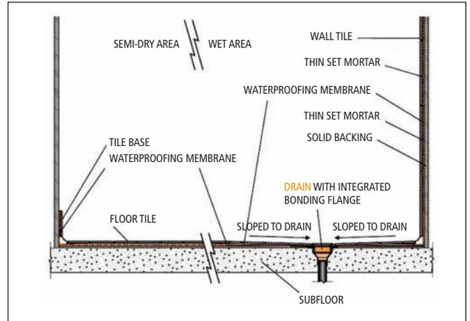
In this situation, the bathroom floor has been raised outside the shower area, with the pre-slope to the drain falling away from the raised bathroom floor. It uses a drain with a bonding flange, surface-applied waterproofing, and small tiles on the shower floor.
