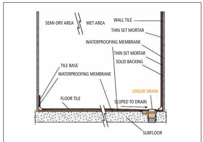
The bathroom floor area has been raised, and it falls away from the shower threshold to a linear drain that has been located on the furthest wall. The single slope allows large tiles on the shower floor.
