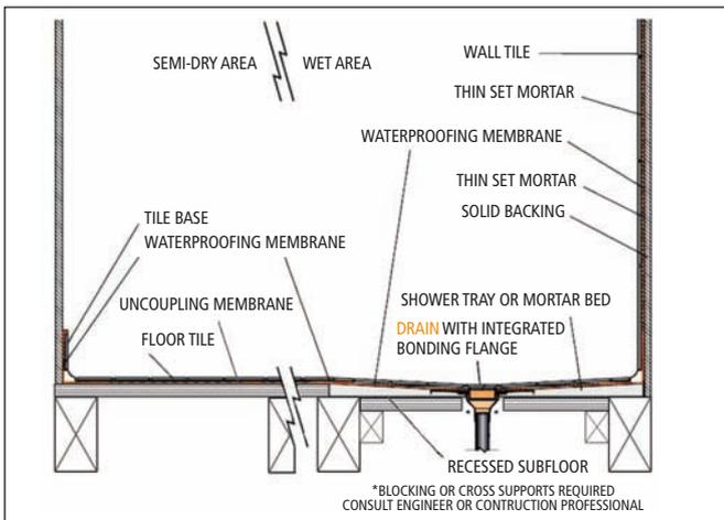
This assembly shows construction over a wood subfloor. The subfloor in the shower area is recessed, which means there is no change in floor height outside of the shower area.
