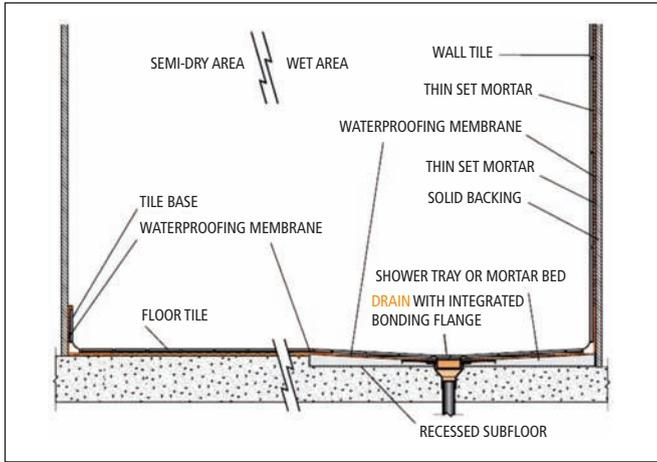
This assembly shows a recessed subfloor in the shower area, using a mortar bed or prefabricated tray over a concrete slab, with a special drain and a bonding flange that tie into the surface-applied waterproofing membrane.
