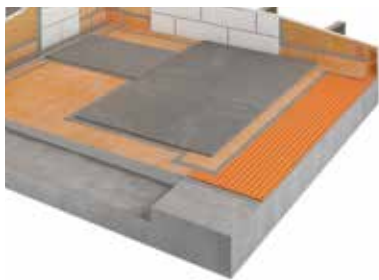
Recessing the Shower Floor
