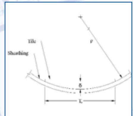
Figure 1. Excessive curvature under a tile due to the bending of the floor sheathing from service loads can produce cracked tile and grout.
