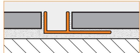
**1.9 Schluter®-DECO-SG** is an anodized aluminum, decorative profile featuring a 1/2" (12.5 mm) wide channel that provides a shadow gap between tile courses or other wall covering. The profile may also be used as a support channel for glass walls, up to a thickness of 3/8" (10 mm). DECO-SG features a trapezoid-perforated anchoring leg that is secured in the bond coat beneath the tile.
