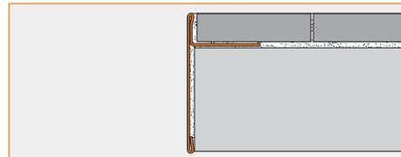
**2.11 Schluter®-SCHIENE-STEP** is a finishing and edging profile for ceramic tile and natural stone installations on countertops, stairs, and tile over tile applications on walls. The profile features a trapezoid-perforated anchoring leg, which is secured in the mortar bond coat beneath the tile. The top of the profile features a vertical wall section that finishes and protects the tile from damage, while the vertical leg covers the edge of the sub-assembly, top of
