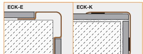
**2.6/2.7 Schluter®-ECK-E/-K** are stainless steel edging profiles for 90° or 135° outside corners of tiled walls that offer excellent edge protection against mechanical stresses; for example, in industrial kitchens and hospitals. In addition, the profiles produce a radiused
