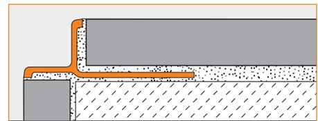
**2.12 Schluter®-INDEC** is an anodized aluminum finishing and edge-protection profile for outside corners of tiled surfaces. It features a trapezoid-perforated anchoring leg that is secured in the mortar bond coat beneath the tile, and the visible surface forms a recessed decorative channel. INDEC can be used as a transition or stop profile to a door or window frame. Matching outside corners are available.
