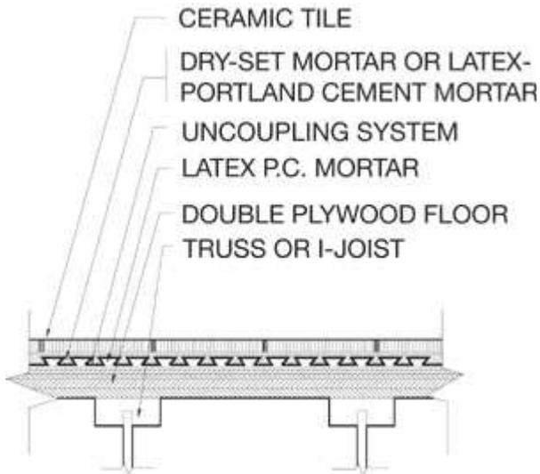
*Floors, Interior Wood Subfloor, 24" o.c. Joist Spacing, with Uncoupling System Latex-Portland Cement*
