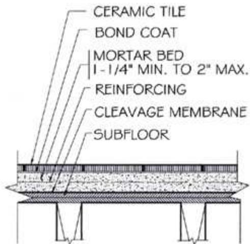
*Floor, Interior Wood Subfloor Cement Mortar*
