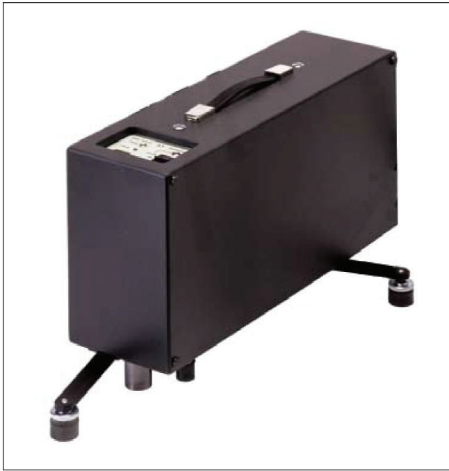
The Type 3207 tapping machine uses five hammers, each weighing 500g and operating at 2Hz, dropping from a height of 40mm, giving an operating frequency of 10Hz. Three extendable legs with rubber feet support the unit during operation.
